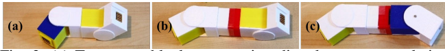
Fig. 3: (a) Two servo blocks connecting directly creates a relative rotation of 90-degree; (b) Extension block can be used to adjust the length of legs; (c) Rotation block can be used to adjust the rotation axis of legs.
