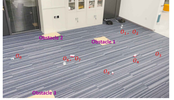
(a) Experimental environment. Eight objects are placed on the floor. The robot duo is tasked to gather them with a tethered net while avoiding obstacles during its navigation.
